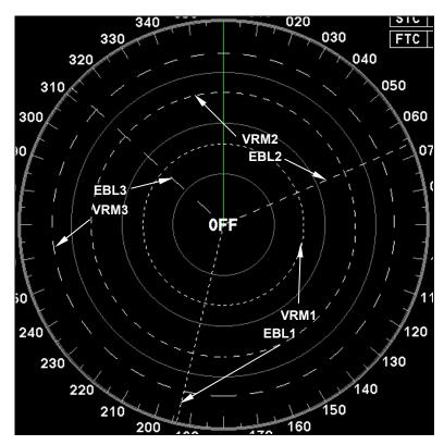
When using multiple EBL/VRMs, the size of the dashes and the distance between dashes allows you to distinguish between the different EBL/VRMs on the display.
